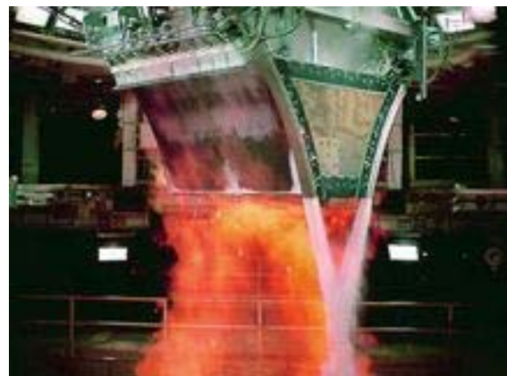
Fig. 12 Photographs of XRS-2200 Boeing Rocketdyne aerospike-engine that will power X-33 (adopted from www.venturestar.com ). The right side photograph shows the engine being tested at its 100% power.
