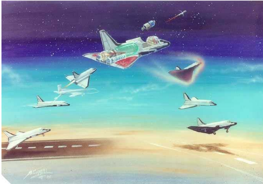
Fig. 8 Sequence of events after Pathfinder launch (Courtesy Pioneer Rocketplane).
